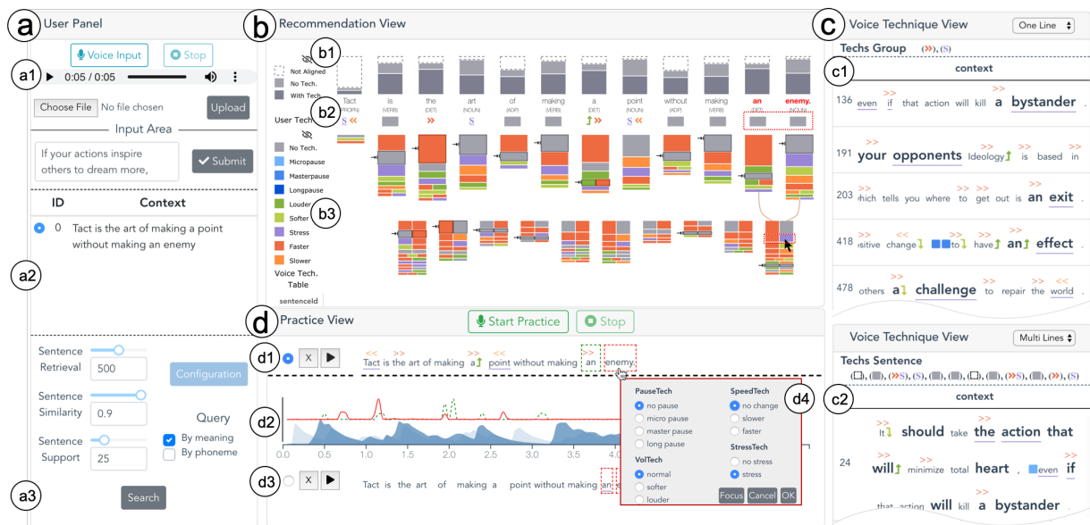
Figure 1: The user interface of VoiceCoach : (a) The user panel allows users to submit a query sentence via audio or text input. (b) The recommendation view presents different levels of recommendation results of modulation combination. (c) The voice technique view enables users to quickly locate and compare the contexts of a specific voice modulation skill in either one-line mode or multi-line mode. (d) The practice view provides users with real-time and quantitative visual feedback to iteratively practice voice modulation skills.
