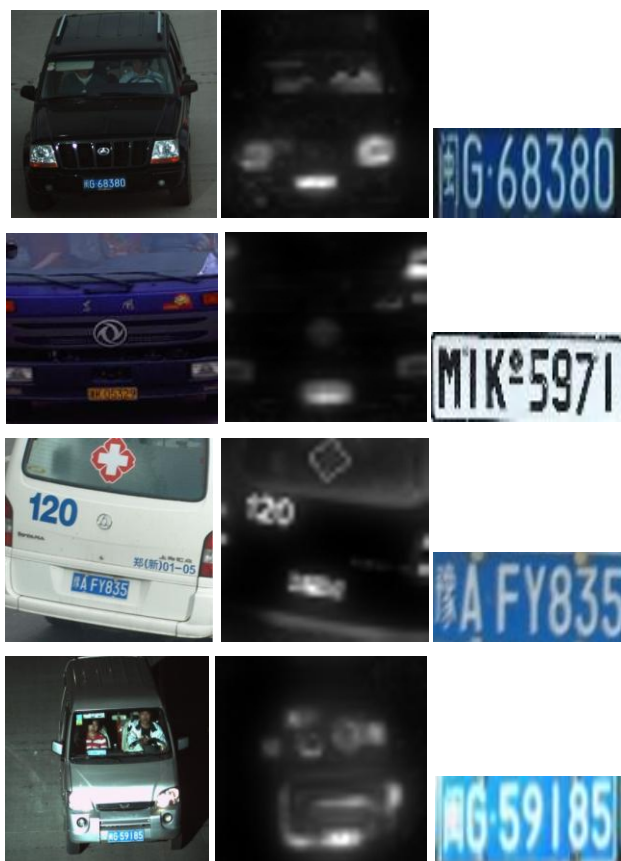
Figure 6. Examples from sample sets and segmentation results. Left:original images,Middle: saliency images, Right: results.
