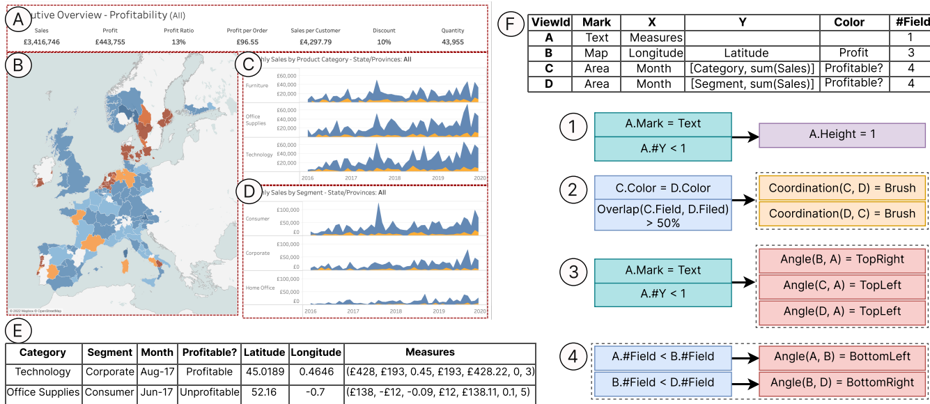
Figure 7. An example dashboard to illustrate identified design rules. The dashboard consists of four views, (A) - (D). Part of the data and the information of each view in the dashboard are shown in two tables, (E) and (F), respectively. In the dashboard, the application of four design rules ((1) - (4)) has been observed. For example, (1) represents that the height of Text view in (A) tends to be 1, and (3) describes that this Text view in (A) tends to be placed on top of other views.
