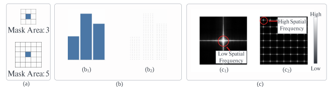
Figure 6: Area-based masking transforms area-based marks from low to high-frequency. (a) Examples of area-based masks with different mask areas. The pixel at the center of the mask remains unchanged, while the adjacent pixels are transformed to match the background color (e.g., white). (b) the effect of applying the area-based masking (Mask area: 5) to a bar chart ( b_1 ) to convert it to its high spatial frequency version ( b_2 ). (c) the frequency domain representations of ( b_1 ) and ( b_2 ).
